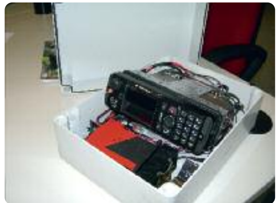
Photo 22 - New alarm system for tube traps (P. Zanghellini - APT Forestry and Wildlife Department Archives)
